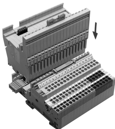
Fig. 24. Installing the manual terminal disconnect module
