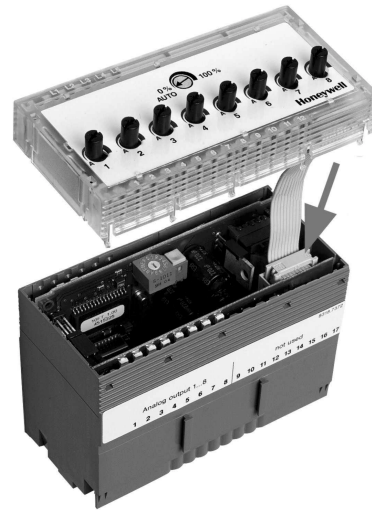
Fig. 21. Manual override connector socket location
